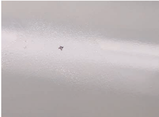
Figure 22: Overpainted oil film which has been applied too thick (no LABS defect) NOTE: There is a camera focus marker in the center
