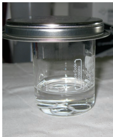
Figure 8: Test specimen in container with solvent
