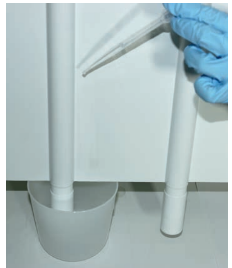
Figure 3: Rinse off tube in cup
