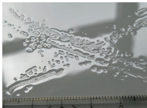
Figure 13: Wetting disturbance after rubbing off (LABS-defect)
