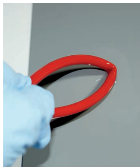
Figure 6: Rub hose / cable in solvent on test plate
