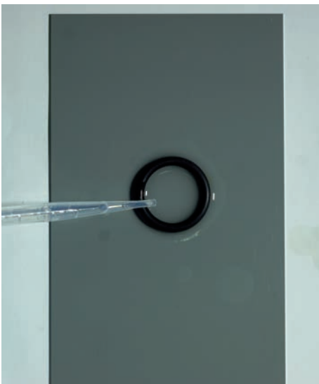
Figure 1: Small test specimen on test plate is rinsed off with solvent
