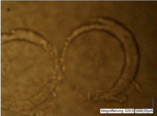
Figure 19b: Solvent edges along O-ring structure (LABS-compliant), image taken with transmitted light
