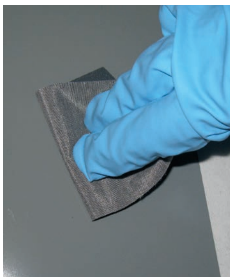
Figure 5: Rub textile on test plate
